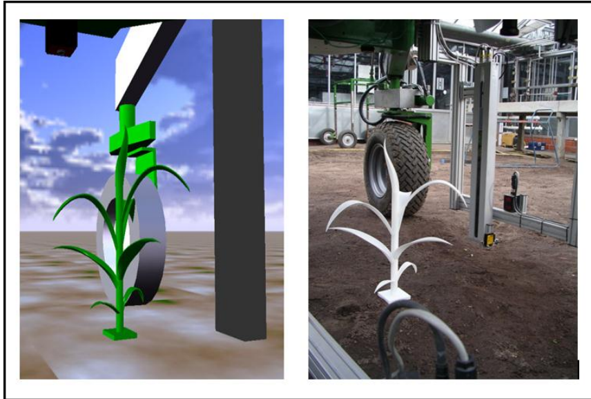
FIGURE 7: Measurement of the artificial plant with virtual (left) and real (right) BoniRob
