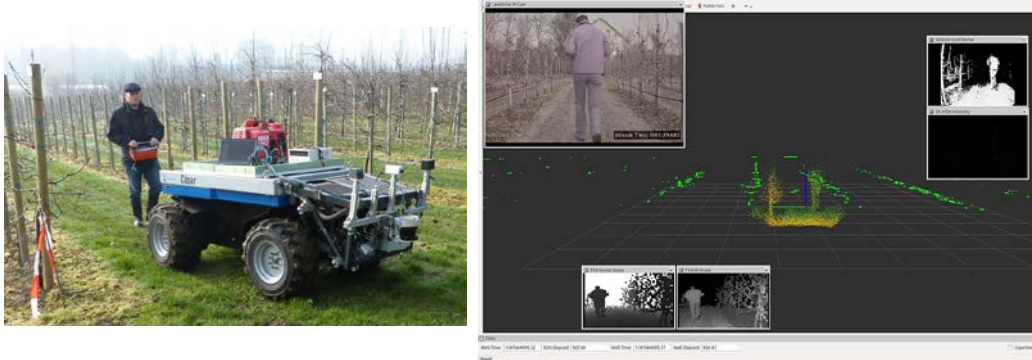
Fig.12. Remote controlled vehicle with mounted sensors and sensor data in Rviz.
